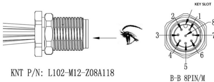
Figure 2.1 Cable Connector on the Lidar Base
