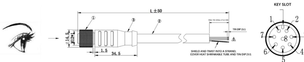
Figure 2.4 C1 Lidar Extension Cable (unit: mm)
