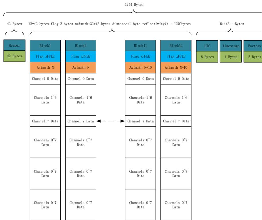
Figure 5.2 Data Format of the Dual Echo Mode
