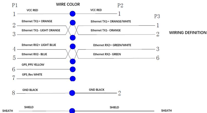
Figure 2.3 Wiring Definition of the Adapter Cable
