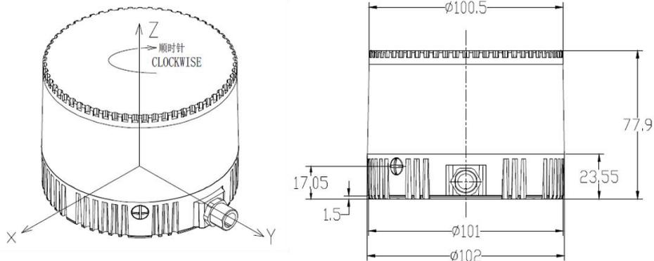
Figure 1.3 C1 Dimensions (unit: mm)
