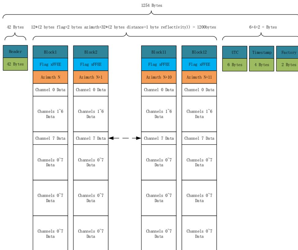
Figure 5.1 Data Format of the Single Echo Mode
