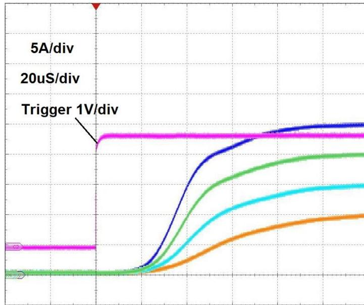
Figure 3. Typical trigger to current delay for Mode 2
